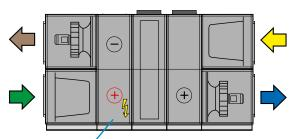
Electrical air heater placed in RX/HC (accessory)
