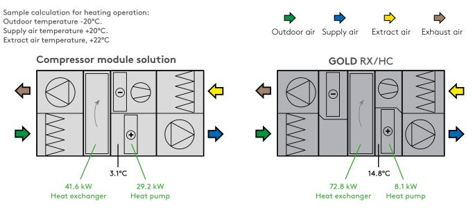
This shows that compressor module solutions largely have to heat the supply air via the heat pump. In the GOLD RX/HC, however, the rotary heat exchanger meets a higher proportion of the power requirement by recovering heating energy from the extract air, which is basically cost-free electrical energy. The heat pump can then top up the remaining proportion of the heating requirement.
