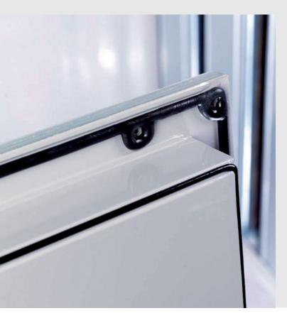
The air handling unit is built on a frame consisting of fiberglass-reinforced polyester U-profiles according to EN 13706 grade E23. Air handling units for outdoor installation are equipped with a roof covering with aluminium finishing strip.
