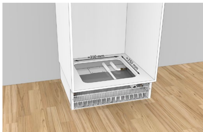
Figure 20. Installed product in cabinet base, where the lower bottom panel has been cut out for good cleaning access.
