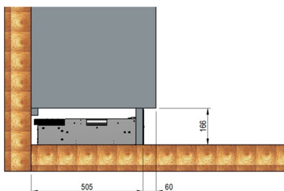
Figure 21. Dimensions - view from the side with CCF mounted in base of 600 cabinet.
