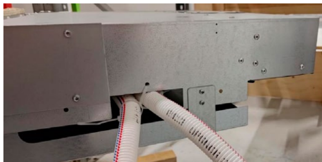
Figure 27. Cut-out for routing the water pipe out from the side of the product.
